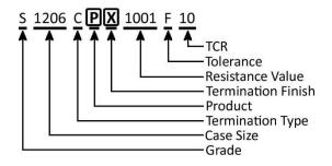
Zero-ohm jumpers have a resistance value code of "000" and do not have tolerance or TCR codes.
